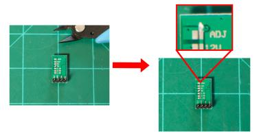
4.) Using a breadboard, multimeter and DC power supply input 8v into the "IN+" pin, "GND" to the GND on your power supply and multimeter, "VO+" to the positive lead on your multimeter. Measure the voltage output of the buck converter. It should read 5v, if it doesn't and your solders look good try cutting the trace deeper as it could still be partially connected.
