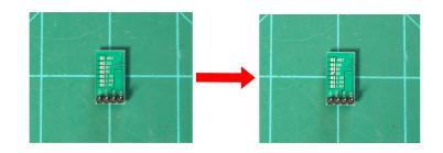
3.) Using a small pair of wire cutters cut the trace just above "ADJ". Make sure its deep enough and removes the top layer of copper.
