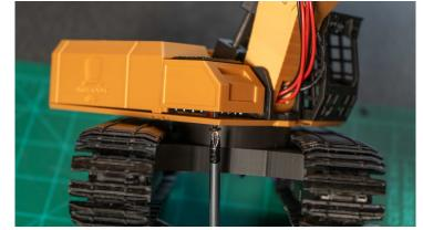
2.) Secure the exhaust to the engine cover using a 2x6mm Screw.
