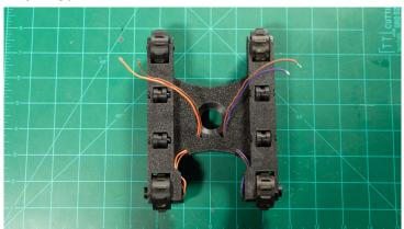
3.) Take x2 3D Printed TPU tracks and gently press them around on the drive gears so they rest in place(they shouldn't be to tight, in fact there might even be a little bit of slack on the bottom of the track).
