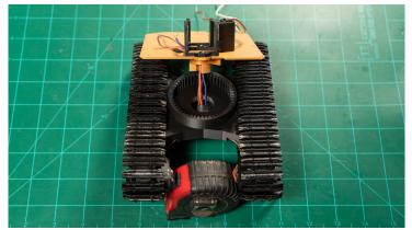
6.) Press the swivel lock into place so that it properly meshes with the lower body and secure with 2x 2x8mm screws.
