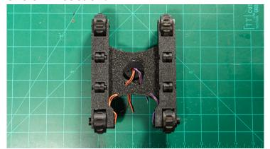
5.) Press the lower body down onto the lower frame while routing the track N20 motor wires up through the tall vertical shaft.
