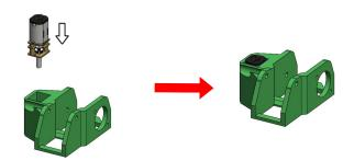
2.) With the motor in place press the 3D printed pinion gear onto the N20 motor from the bottom using just your hand and then if required either a vice or by gently tapping with a hammer the rest of the way on.
