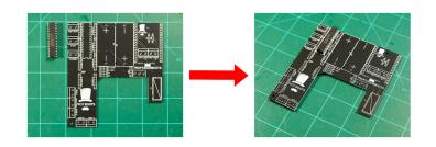
Solder on a completed 5v buck converter.
