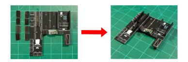
Solder all 10 terminal blocks on, verify each block is facing the correct direction by cross referencing the photos below. Where they are stacked beside each other it helps to lock them together first.
