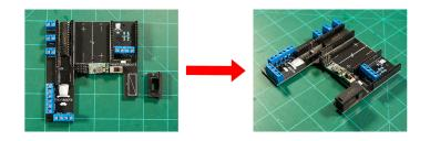
Solder 2 CR123A Battery holders on making sure to match the positive(+) symbols of the holders to the positive(+) symbols of the ProfBoots PCB.
