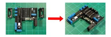
With everything soldered flip the board over and trim any pins that stick out excessively.
