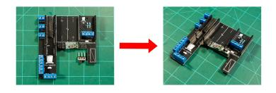
Solder on the fuse holder so the cover swings back towards the ESP32 development board.
