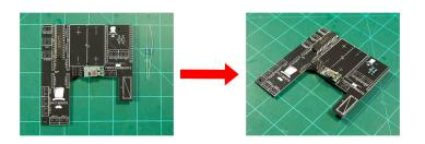
Solder 2 sets of 15pin female headers onto where the ESP32 development board will mount.
