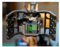
15.) Power up the excavator and make sure you have full range of motion on the claw using the "Triangle" and "X" buttons on the right side of the controller. If not power down and adjust the servo horn placement.
