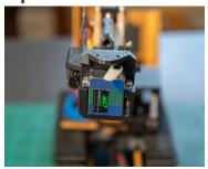
13.) Secure both the left and right claw arms onto the servo holder using 42.6x8mm screws. Taking care to mesh the gears correctly.
