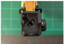
9.) Route the servo wires through the center and then out through the cutout in the dipper.
