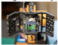
14.) Run the 3D Printed "Claw Servo Push Link" from the left arm(secured via a 2.6x6mm screw to the 2-3rd hole from the center of the servo horn using a smaller 2x6mm screw.
