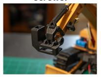
5.) Insert the 12v 100RPM N20 motor into the rotating claw attacher. Route the wires back down the arm into either terminal block "aux-atch" or "thumb" depending on your controller layout preference after stripping back the wires 1cm.
