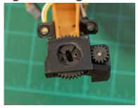
8.) First align the center cutouts on the servo holder, output gear, and attacher then Secure the "Rotating Claw Servo Holder" to the output gear using 2
