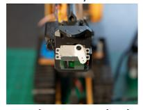
12.) Press the servo wire into the provided channel along the back of the servo holder and then press the servo into place, putting the servo horn on the right side of the servo holder if looking from the front. Lock the servo into place using the two silver screws
