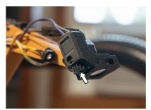
7.) Slide the 3D printed "Output Gear for Claw Rotation" into the rotating claw attacher with the cutouts on the gear facing down.
