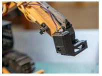
6.) Press the 3D printed "Pinion Gear for Claw Rotation Motor" onto the shaft of the N20 motor.
