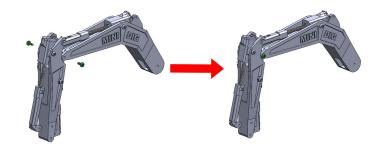
4.) Attach the dipper to the N20 motor mounted to the main booms push rod using 2 2x6mm screws.
