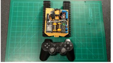
4.) Verify that the motors move in the correct direction by pressing the front triggers and bumpers. The bumpers should be forward and triggers should be reverse. The pivot should swing left and right via the left joystick left and right.
