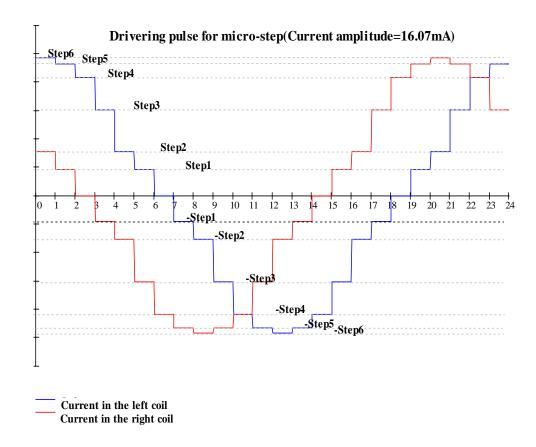
In general the peak amplitude should be between 12.9mA and 16.07mA.
