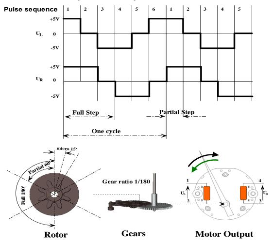
In order to make the motor run more stablely and reduce its noise, micro stepping technology is recommended. The micro pulse sequence which is more precise and near to sine wave, which could drive motor with 1/12° micro step of the pointer. The diagram is as following:
